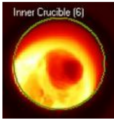
Figure 13: Thermal imaging: industrial induction melting
